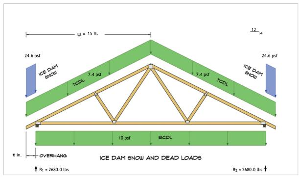
$$\begin{split} R_1 &= D + S = 2556.8 \text{ lbs} + 123.2 \text{ lbs} \\ R_2 &= D + S = 2556.8 \text{ lbs} + 123.2 \text{ lbs} \end{split}$$
