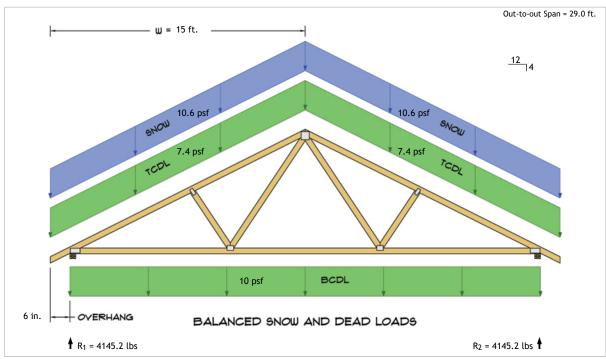
$$\begin{split} R_1 &= D + S = 2556.8 \text{ lbs} + 1588.4 \text{ lbs} \\ R_2 &= D + S = 2556.8 \text{ lbs} + 1588.4 \text{ lbs} \end{split}$$
