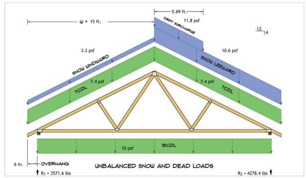
$R_1 = D + S = 2556.8 \text{ lbs} + 1014.8 \text{ lbs}$  $R_2 = D + S = 2556.8 \text{ lbs} + 1721.6 \text{ lbs}$
