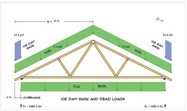
$$\begin{split} R_1 &= D + S = 2556.8 \text{ lbs} + 123.2 \text{ lbs} \\ R_2 &= D + S = 2556.8 \text{ lbs} + 123.2 \text{ lbs} \end{split}$$
