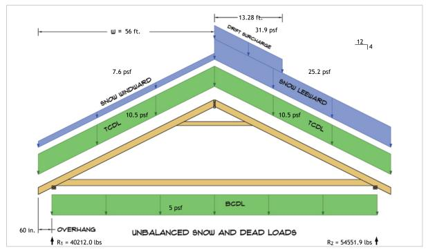
$R_1 = D + S = 20287.0 \text{ lbs} + 19925.0 \text{ lbs}$  $R_2 = D + S = 20287.0 \text{ lbs} + 34264.9 \text{ lbs}$
