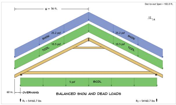
$$\begin{split} R_1 &= D + S = 20287.0 \text{ lbs} + 33873.7 \text{ lbs} \\ R_2 &= D + S = 20287.0 \text{ lbs} + 33873.7 \text{ lbs} \end{split}$$
