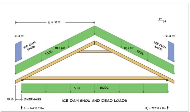
$R_1 = D + S = 20287.0 \text{ lbs} + 6451.2 \text{ lbs}$  $R_2 = D + S = 20287.0 \text{ lbs} + 6451.2 \text{ lbs}$
