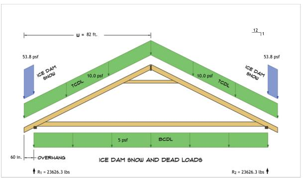
$R_1 = D + S = 19325.5 \text{ lbs} + 4300.8 \text{ lbs}$  $R_2 = D + S = 19325.5 \text{ lbs} + 4300.8 \text{ lbs}$
