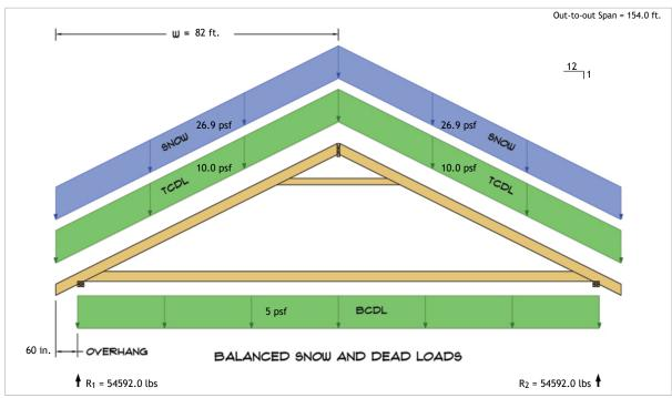
$$\begin{split} R_1 &= D + S = 19325.5 \text{ lbs} + 35266.6 \text{ lbs} \\ R_2 &= D + S = 19325.5 \text{ lbs} + 35266.6 \text{ lbs} \end{split}$$
