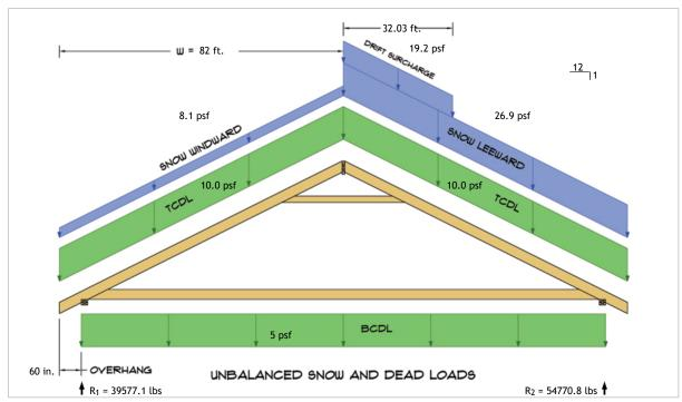
$R_1 = D + S = 19325.5 \text{ lbs} + 20251.6 \text{ lbs}$  $R_2 = D + S = 19325.5 \text{ lbs} + 35445.3 \text{ lbs}$
