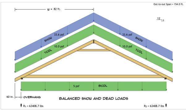
$$\begin{split} R_1 &= D + S = 19325.5 \text{ lbs} + 44083.2 \text{ lbs} \\ R_2 &= D + S = 19325.5 \text{ lbs} + 44083.2 \text{ lbs} \end{split}$$
