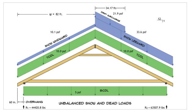
$R_1 = D + S = 19325.5 \text{ lbs} + 25095.3 \text{ lbs}$  $R_2 = D + S = 19325.5 \text{ lbs} + 44182.4 \text{ lbs}$
