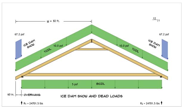
$R_1 = D + S = 19325.5 \text{ lbs} + 5376.0 \text{ lbs}$  $R_2 = D + S = 19325.5 \text{ lbs} + 5376.0 \text{ lbs}$
