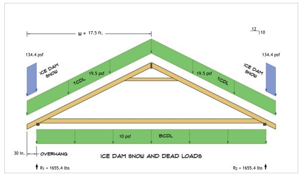
$\begin{aligned} R_1 &= D + S = 983.4 \text{ lbs} + 672.0 \text{ lbs} \\ R_2 &= D + S = 983.4 \text{ lbs} + 672.0 \text{ lbs} \end{aligned}$
