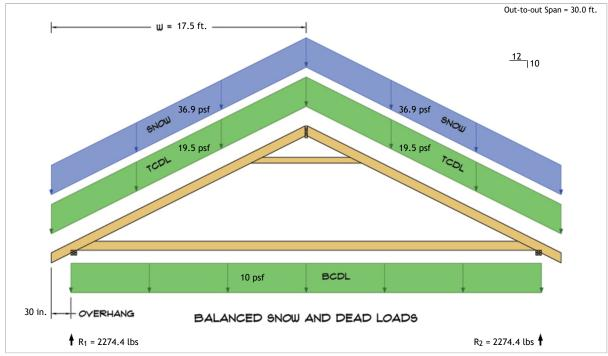
$R_1 = D + S = 983.4 \text{ lbs} + 1291.0 \text{ lbs}$  $R_2 = D + S = 983.4 \text{ lbs} + 1291.0 \text{ lbs}$
