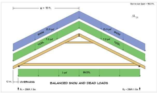
$\begin{aligned} R_1 &= D + S = 797.1 \text{ lbs} + 2072.0 \text{ lbs} \\ R_2 &= D + S = 797.1 \text{ lbs} + 2072.0 \text{ lbs} \end{aligned}$
