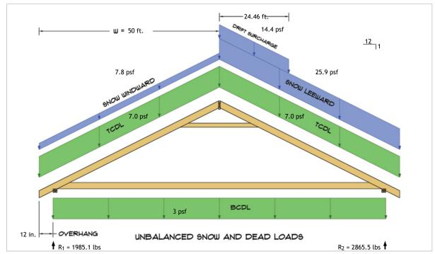
$R_1 = D + S = 797.1 \text{ lbs} + 1187.9 \text{ lbs}$  $R_2 = D + S = 797.1 \text{ lbs} + 2068.3 \text{ lbs}$
