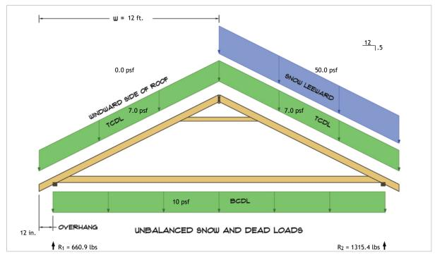
$R_1 = D + S = 388.1 \text{ lbs} + 272.7 \text{ lbs}$  $R_2 = D + S = 388.1 \text{ lbs} + 927.3 \text{ lbs}$
