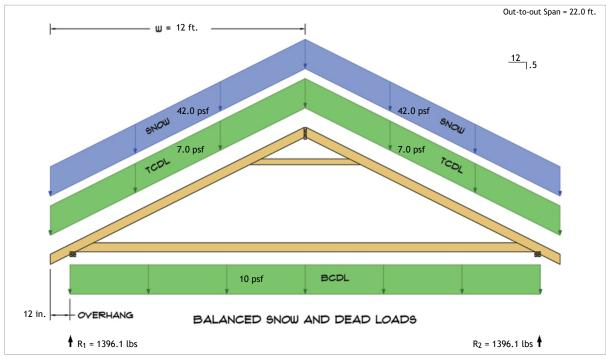
$R_1 = D + S = 388.1 \text{ lbs} + 1008.0 \text{ lbs}$  $R_2 = D + S = 388.1 \text{ lbs} + 1008.0 \text{ lbs}$
