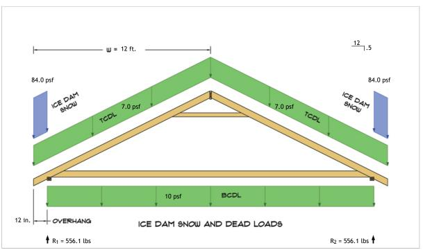
$R_1 = D + S = 388.1 \text{ lbs} + 168.0 \text{ lbs}$  $R_2 = D + S = 388.1 \text{ lbs} + 168.0 \text{ lbs}$
