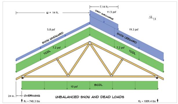
$R_1 = D + S = 442.0 \text{ lbs} + 298.2 \text{ lbs}$  $R_2 = D + S = 442.0 \text{ lbs} + 567.4 \text{ lbs}$
