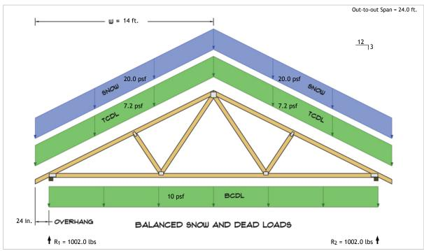
$$\begin{split} R_1 &= D + S = 442.0 \text{ lbs} + 560.0 \text{ lbs} \\ R_2 &= D + S = 442.0 \text{ lbs} + 560.0 \text{ lbs} \end{split}$$
