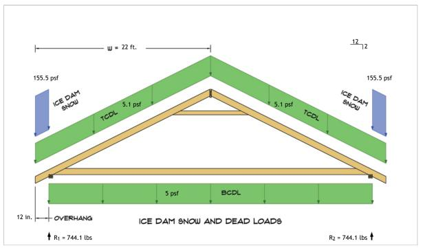
$$\begin{split} R_1 &= D + S = 433.0 \text{ lbs} + 311.1 \text{ lbs} \\ R_2 &= D + S = 433.0 \text{ lbs} + 311.1 \text{ lbs} \end{split}$$
