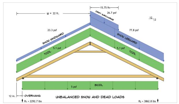
$R_1 = D + S = 433.0 \text{ lbs} + 1859.7 \text{ lbs}$  $R_2 = D + S = 433.0 \text{ lbs} + 3429.7 \text{ lbs}$
