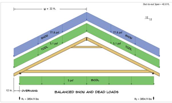
$\begin{aligned} R_1 &= D + S = 433.0 \text{ lbs} + 3421.9 \text{ lbs} \\ R_2 &= D + S = 433.0 \text{ lbs} + 3421.9 \text{ lbs} \end{aligned}$
