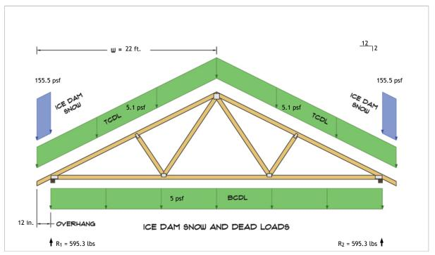
$\begin{aligned} R_1 &= D + S = 346.4 \text{ lbs} + 248.9 \text{ lbs} \\ R_2 &= D + S = 346.4 \text{ lbs} + 248.9 \text{ lbs} \end{aligned}$
