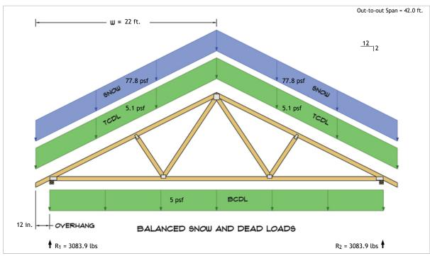
$$\begin{split} R_1 &= D + S = 346.4 \text{ lbs} + 2737.5 \text{ lbs} \\ R_2 &= D + S = 346.4 \text{ lbs} + 2737.5 \text{ lbs} \end{split}$$
