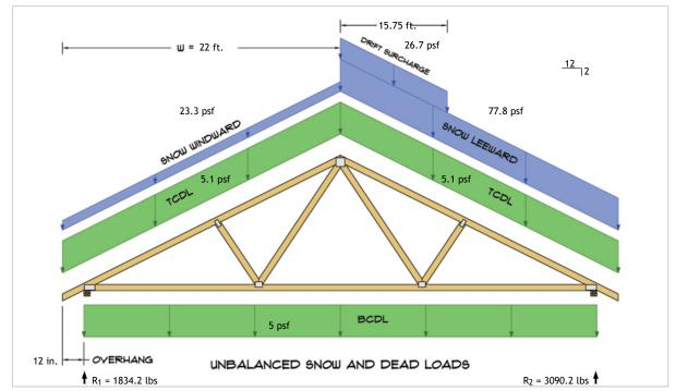
$R_1 = D + S = 346.4 \text{ lbs} + 1487.8 \text{ lbs}$  $R_2 = D + S = 346.4 \text{ lbs} + 2743.8 \text{ lbs}$
