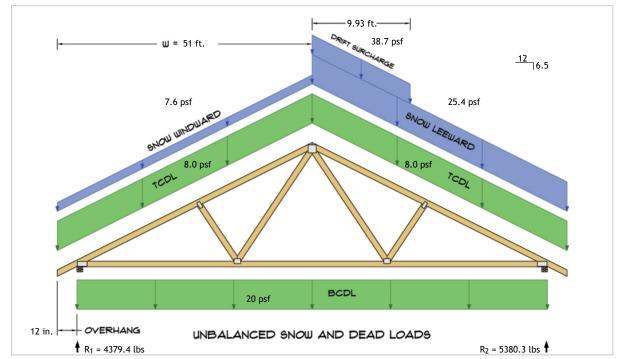
$R_1 = D + S = 2812.0 \text{ lbs} + 1567.4 \text{ lbs}$  $R_2 = D + S = 2812.0 \text{ lbs} + 2568.2 \text{ lbs}$
