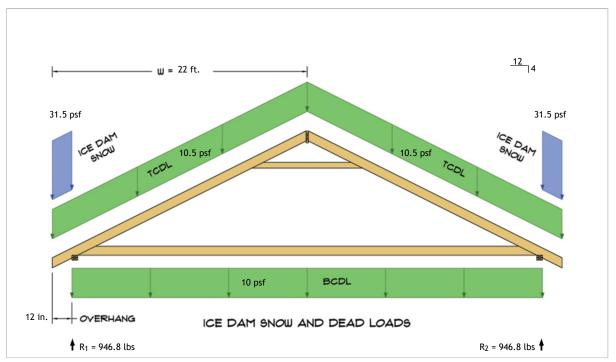
$$\begin{split} R_1 &= D + S = 883.8 \text{ lbs} + 63.0 \text{ lbs} \\ R_2 &= D + S = 883.8 \text{ lbs} + 63.0 \text{ lbs} \end{split}$$
