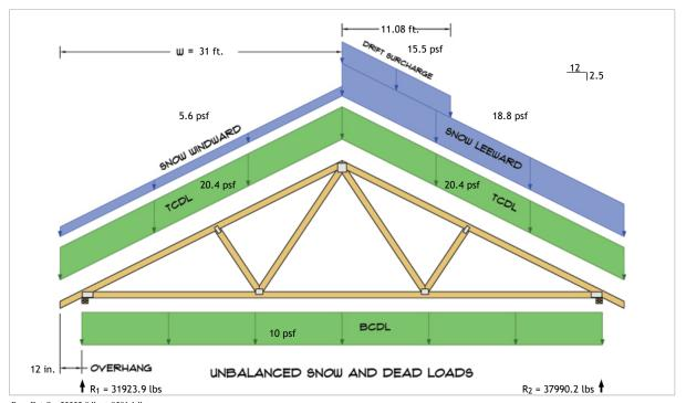
$R_1 = D + S = 23332.8 \text{ lbs} + 8591.1 \text{ lbs}$  $R_2 = D + S = 23332.8 \text{ lbs} + 14657.4 \text{ lbs}$
