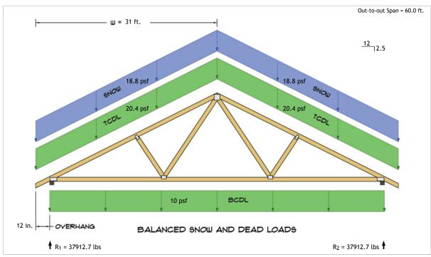
$$\begin{split} R_1 &= D + S = 23332.8 \text{ lbs} + 14579.9 \text{ lbs} \\ R_2 &= D + S = 23332.8 \text{ lbs} + 14579.9 \text{ lbs} \end{split}$$
