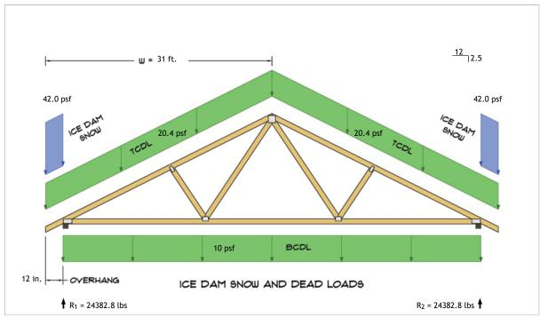
$$\begin{split} R_1 &= D + S = 23332.8 \text{ lbs} + 1050.0 \text{ lbs} \\ R_2 &= D + S = 23332.8 \text{ lbs} + 1050.0 \text{ lbs} \end{split}$$
