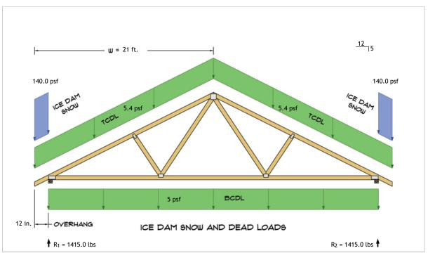
$R_1 = D + S = 855.0 \text{ lbs} + 560.0 \text{ lbs}$  $R_2 = D + S = 855.0 \text{ lbs} + 560.0 \text{ lbs}$
