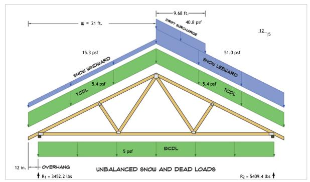
$R_1 = D + S = 855.0 \text{ lbs} + 2597.2 \text{ lbs}$  $R_2 = D + S = 855.0 \text{ lbs} + 4554.4 \text{ lbs}$
