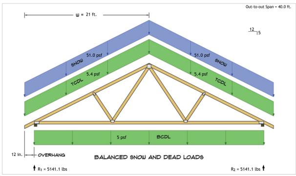
$$\begin{split} R_1 &= D + S = 855.0 \text{ lbs} + 4286.1 \text{ lbs} \\ R_2 &= D + S = 855.0 \text{ lbs} + 4286.1 \text{ lbs} \end{split}$$
