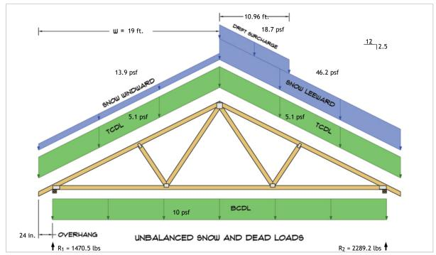
$R_1 = D + S = 534.1 \text{ lbs} + 936.4 \text{ lbs}$  $R_2 = D + S = 534.1 \text{ lbs} + 1755.1 \text{ lbs}$
