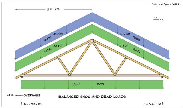
$\begin{aligned} R_1 &= D + S = 534.1 \text{ lbs} + 1755.6 \text{ lbs} \\ R_2 &= D + S = 534.1 \text{ lbs} + 1755.6 \text{ lbs} \end{aligned}$
