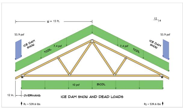
$R_1 = D + S = 431.8 \text{ lbs} + 107.8 \text{ lbs}$  $R_2 = D + S = 431.8 \text{ lbs} + 107.8 \text{ lbs}$
