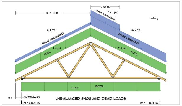
$R_1 = D + S = 431.8 \text{ lbs} + 403.7 \text{ lbs}$  $R_2 = D + S = 431.8 \text{ lbs} + 736.7 \text{ lbs}$
