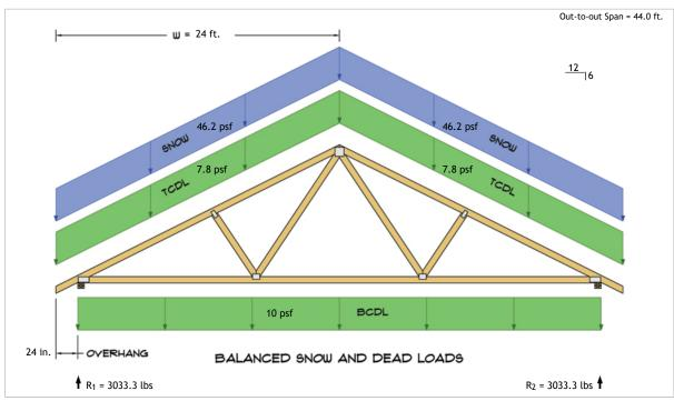
$\begin{aligned} R_1 &= D + S = 815.7 \text{ lbs} + 2217.6 \text{ lbs} \\ R_2 &= D + S = 815.7 \text{ lbs} + 2217.6 \text{ lbs} \end{aligned}$
