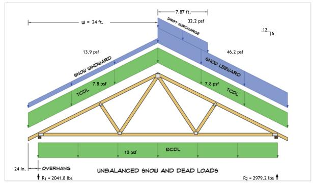
$R_1 = D + S = 815.7 \text{ lbs} + 1226.1 \text{ lbs}$  $R_2 = D + S = 815.7 \text{ lbs} + 2163.5 \text{ lbs}$
