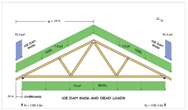
$$\begin{split} R_1 &= D + S = 815.7 \text{ lbs} + 369.6 \text{ lbs} \\ R_2 &= D + S = 815.7 \text{ lbs} + 369.6 \text{ lbs} \end{split}$$
