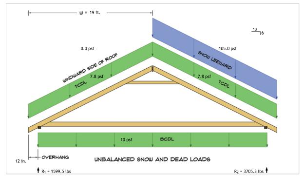
$\begin{aligned} R_1 &= D + S = 657.4 \text{ lbs} + 942.1 \text{ lbs} \\ R_2 &= D + S = 657.4 \text{ lbs} + 3047.9 \text{ lbs} \end{aligned}$
