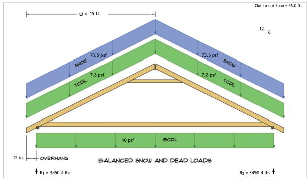
$R_1 = D + S = 657.4 \text{ lbs} + 2793.0 \text{ lbs}$  $R_2 = D + S = 657.4 \text{ lbs} + 2793.0 \text{ lbs}$
