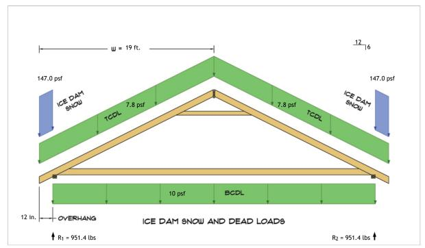
$$\begin{split} R_1 &= D + S = 657.4 \text{ lbs} + 294.0 \text{ lbs} \\ R_2 &= D + S = 657.4 \text{ lbs} + 294.0 \text{ lbs} \end{split}$$
