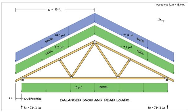
$$\begin{split} R_1 &= D + S = 324.3 \text{ lbs} + 400.0 \text{ lbs} \\ R_2 &= D + S = 324.3 \text{ lbs} + 400.0 \text{ lbs} \end{split}$$
