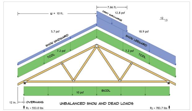
$R_1 = D + S = 324.3 \text{ lbs} + 228.7 \text{ lbs}$  $R_2 = D + S = 324.3 \text{ lbs} + 459.4 \text{ lbs}$
