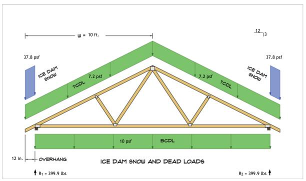
$\begin{aligned} R_1 &= D + S = 324.3 \text{ lbs} + 75.6 \text{ lbs} \\ R_2 &= D + S = 324.3 \text{ lbs} + 75.6 \text{ lbs} \end{aligned}$
