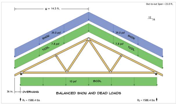
$$\begin{aligned} R_1 &= D + S = 457.0 \text{ lbs} + 1131.4 \text{ lbs} \\ R_2 &= D + S = 457.0 \text{ lbs} + 1131.4 \text{ lbs} \end{aligned}$$
