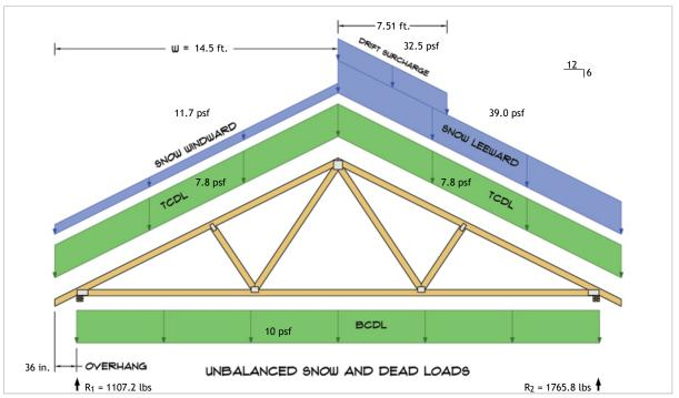
$R_1 = D + S = 457.0 \text{ lbs} + 650.2 \text{ lbs}$  $R_2 = D + S = 457.0 \text{ lbs} + 1308.9 \text{ lbs}$
