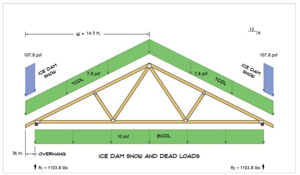
$$\begin{split} R_1 &= D + S = 457.0 \text{ lbs} + 646.8 \text{ lbs} \\ R_2 &= D + S = 457.0 \text{ lbs} + 646.8 \text{ lbs} \end{split}$$
