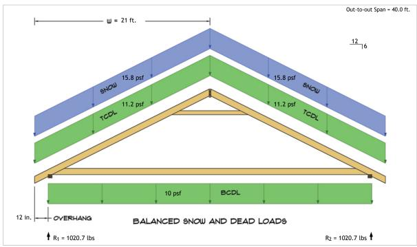
$\begin{aligned} R_1 &= D + S = 579.7 \text{ lbs} + 441.0 \text{ lbs} \\ R_2 &= D + S = 579.7 \text{ lbs} + 441.0 \text{ lbs} \end{aligned}$
