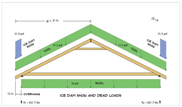
$\begin{aligned} R_1 &= D + S = 579.7 \text{ lbs} + 42.0 \text{ lbs} \\ R_2 &= D + S = 579.7 \text{ lbs} + 42.0 \text{ lbs} \end{aligned}$
