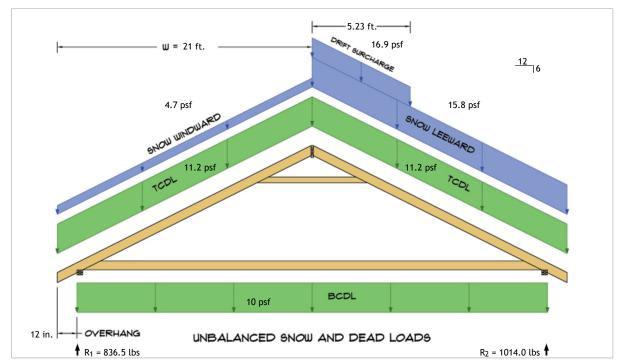
$R_1 = D + S = 579.7 \text{ lbs} + 256.8 \text{ lbs}$  $R_2 = D + S = 579.7 \text{ lbs} + 434.2 \text{ lbs}$
