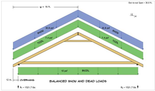
$R_1 = D + S = 536.1 \text{ lbs} + 985.6 \text{ lbs}$  $R_2 = D + S = 536.1 \text{ lbs} + 985.6 \text{ lbs}$
