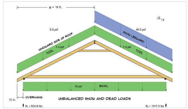
$R_1 = D + S = 536.1 \text{ lbs} + 298.7 \text{ lbs}$  $R_2 = D + S = 536.1 \text{ lbs} + 981.3 \text{ lbs}$
