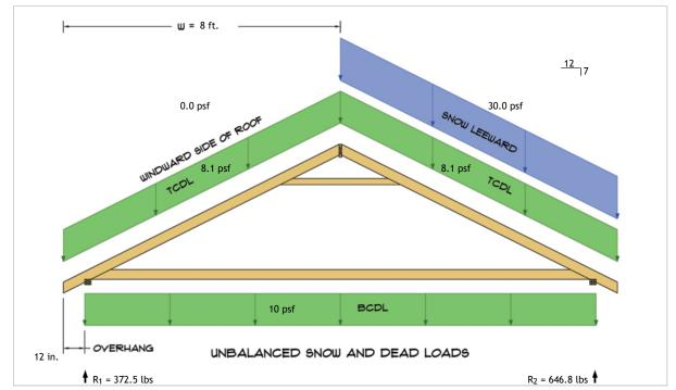
$R_1 = D + S = 269.7 \text{ lbs} + 102.9 \text{ lbs}$  $R_2 = D + S = 269.7 \text{ lbs} + 377.1 \text{ lbs}$
