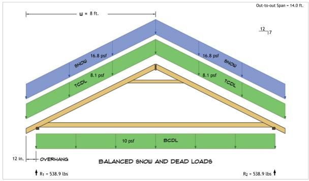
$R_1 = D + S = 269.7 \text{ lbs} + 269.3 \text{ lbs}$  $R_2 = D + S = 269.7 \text{ lbs} + 269.3 \text{ lbs}$
