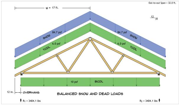
$R_1 = D + S = 524.3 \text{ lbs} + 2879.8 \text{ lbs}$  $R_2 = D + S = 524.3 \text{ lbs} + 2879.8 \text{ lbs}$
