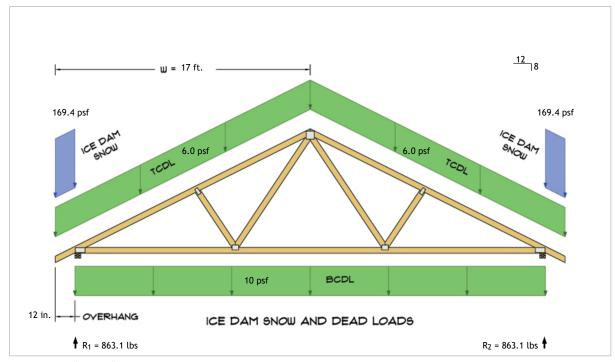
$\begin{aligned} R_1 &= D + S = 524.3 \text{ lbs} + 338.8 \text{ lbs} \\ R_2 &= D + S = 524.3 \text{ lbs} + 338.8 \text{ lbs} \end{aligned}$
