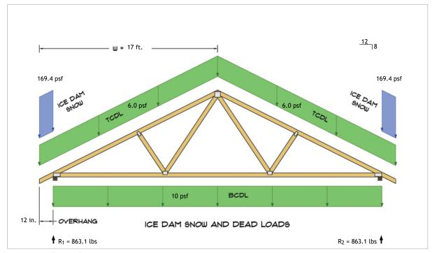
$R_1 = D + S = 524.3 \text{ lbs} + 338.8 \text{ lbs}$  $R_2 = D + S = 524.3 \text{ lbs} + 338.8 \text{ lbs}$
