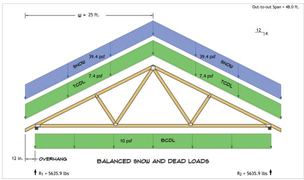
$$\begin{split} R_1 &= D + S = 1697.9 \text{ lbs} + 3938.1 \text{ lbs} \\ R_2 &= D + S = 1697.9 \text{ lbs} + 3938.1 \text{ lbs} \end{split}$$
