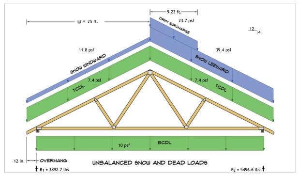
$R_1 = D + S = 1697.9 \text{ lbs} + 2194.8 \text{ lbs}$  $R_2 = D + S = 1697.9 \text{ lbs} + 3798.8 \text{ lbs}$
