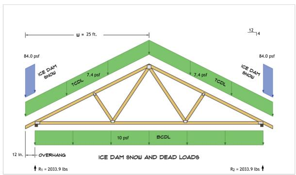
$R_1 = D + S = 1697.9 \text{ lbs} + 336.0 \text{ lbs}$  $R_2 = D + S = 1697.9 \text{ lbs} + 336.0 \text{ lbs}$
