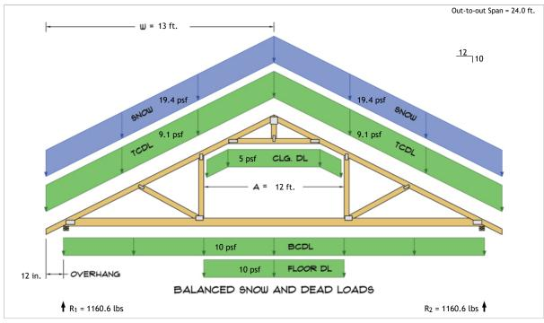
$R_1 = D + S = 656.9 \text{ lbs} + 503.7 \text{ lbs}$  $R_2 = D + S = 656.9 \text{ lbs} + 503.7 \text{ lbs}$
