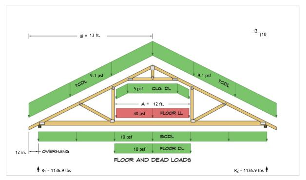
$R_1 = D + L = 656.9 \text{ lbs} + 480.0 \text{ lbs} \\ R_2 = D + L = 656.9 \text{ lbs} + 480.0 \text{ lbs}$
