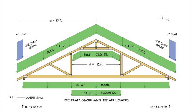
$\begin{aligned} R_1 &= D + S = 656.9 \text{ lbs} + 154.0 \text{ lbs} \\ R_2 &= D + S = 656.9 \text{ lbs} + 154.0 \text{ lbs} \end{aligned}$
