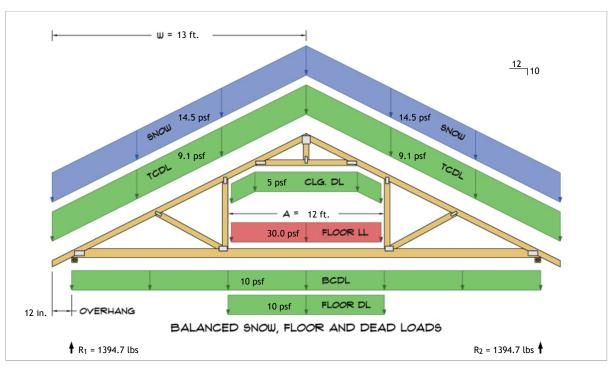
$$\begin{split} R_1 &= D + 0.75L + 0.75S = 656.9 \text{ lbs} + 360.0 \text{ lbs} + 377.8 \text{ lbs} \\ R_2 &= D + 0.75L + 0.75S = 656.9 \text{ lbs} + 360.0 \text{ lbs} + 377.8 \text{ lbs} \end{split}$$
