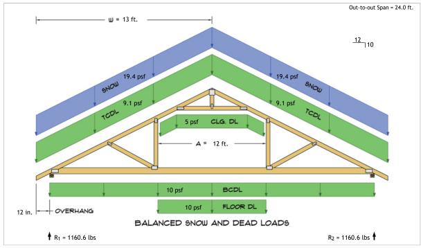
$R_1 = D + S = 656.9 \text{ lbs} + 503.7 \text{ lbs}$  $R_2 = D + S = 656.9 \text{ lbs} + 503.7 \text{ lbs}$
