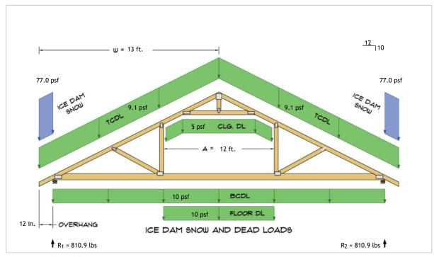
$\begin{aligned} R_1 &= D + S = 656.9 \text{ lbs} + 154.0 \text{ lbs} \\ R_2 &= D + S = 656.9 \text{ lbs} + 154.0 \text{ lbs} \end{aligned}$
