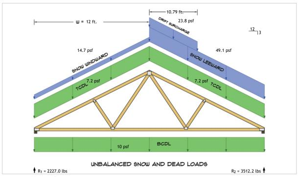
$R_1 = D + S = 826.3 \text{ lbs} + 1400.7 \text{ lbs} \\ R_2 = D + S = 826.3 \text{ lbs} + 2685.8 \text{ lbs}$
