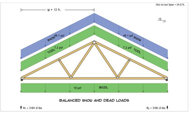
$R_1 = D + S = 826.3 \text{ lbs} + 2354.7 \text{ lbs}$  $R_2 = D + S = 826.3 \text{ lbs} + 2354.7 \text{ lbs}$
