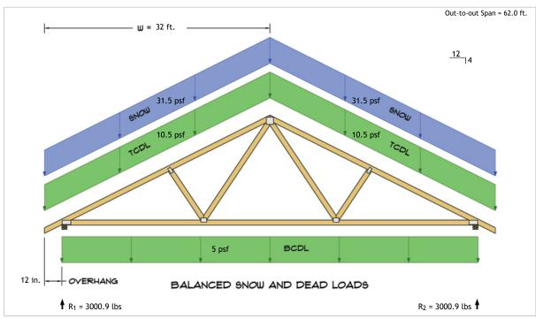
$\begin{aligned} R_1 &= D + S = 984.6 \text{ lbs} + 2016.3 \text{ lbs} \\ R_2 &= D + S = 984.6 \text{ lbs} + 2016.3 \text{ lbs} \end{aligned}$
