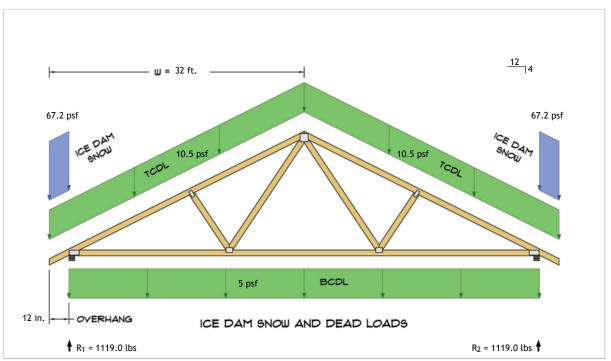
$R_1 = D + S = 984.6 \text{ lbs} + 134.4 \text{ lbs}$  $R_2 = D + S = 984.6 \text{ lbs} + 134.4 \text{ lbs}$
