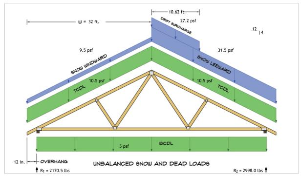
$R_1 = D + S = 984.6 \text{ lbs} + 1185.9 \text{ lbs}$  $R_2 = D + S = 984.6 \text{ lbs} + 2013.4 \text{ lbs}$
