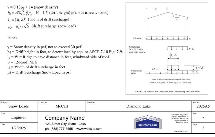
$$\begin{aligned} p_{\text{windward}} &= 0.3 \, \text{ps} = (0.3)(67.8) = 20.3 \, \text{psf} \\ p_{\text{leeward}} &= p_{\text{s}} = 67.8 \, \text{psf} \end{aligned}$$
