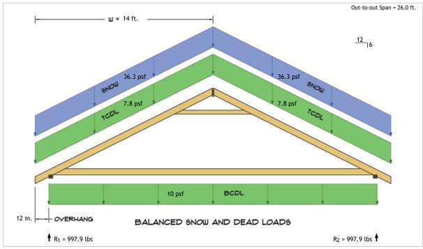
$R_1 = D + S = 319.4 \text{ lbs} + 678.5 \text{ lbs}$  $R_2 = D + S = 319.4 \text{ lbs} + 678.5 \text{ lbs}$
