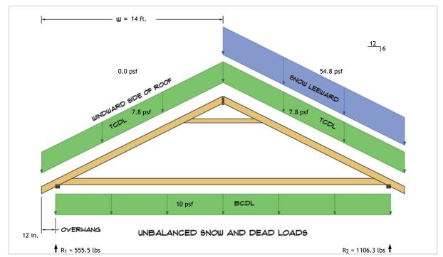
$R_1 = D + S = 319.4 \text{ lbs} + 236.1 \text{ lbs}$  $R_2 = D + S = 319.4 \text{ lbs} + 786.9 \text{ lbs}$
