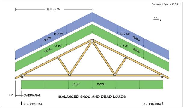
$$\begin{split} R_1 &= D + S = 1035.0 \text{ lbs} + 2772.0 \text{ lbs} \\ R_2 &= D + S = 1035.0 \text{ lbs} + 2772.0 \text{ lbs} \end{split}$$
