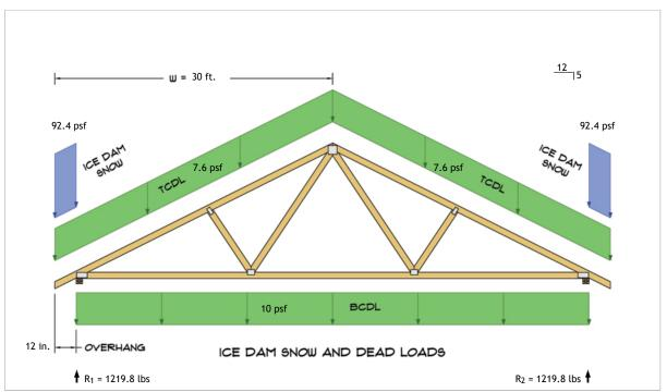
$R_1 = D + S = 1035.0 \text{ lbs} + 184.8 \text{ lbs}$  $R_2 = D + S = 1035.0 \text{ lbs} + 184.8 \text{ lbs}$
