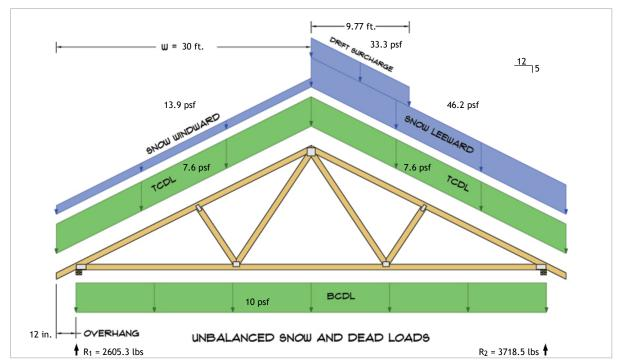
$R_1 = D + S = 1035.0 \text{ lbs} + 1570.3 \text{ lbs}$  $R_2 = D + S = 1035.0 \text{ lbs} + 2683.5 \text{ lbs}$
