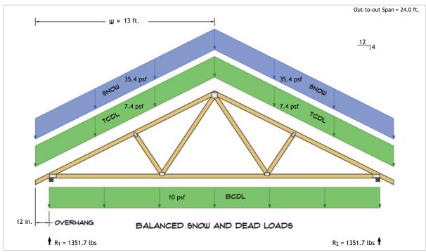
$$\begin{split} R_1 &= D + S = 431.8 \text{ lbs} + 919.9 \text{ lbs} \\ R_2 &= D + S = 431.8 \text{ lbs} + 919.9 \text{ lbs} \end{split}$$
