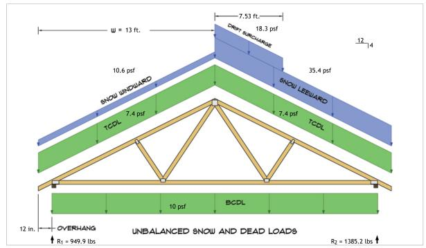
$R_1 = D + S = 431.8 \text{ lbs} + 518.1 \text{ lbs}$  $R_2 = D + S = 431.8 \text{ lbs} + 953.4 \text{ lbs}$
