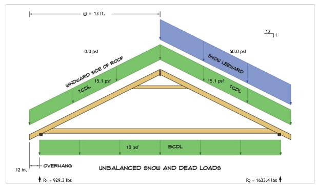
$R_1 = D + S = 631.4 \text{ lbs} + 297.9 \text{ lbs}$  $R_2 = D + S = 631.4 \text{ lbs} + 1002.1 \text{ lbs}$
