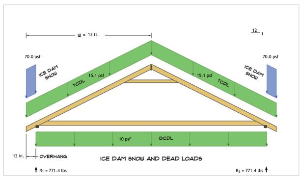
$R_1 = D + S = 631.4 \text{ lbs} + 140.0 \text{ lbs}$  $R_2 = D + S = 631.4 \text{ lbs} + 140.0 \text{ lbs}$
