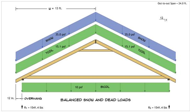
$R_1 = D + S = 631.4 \text{ lbs} + 910.0 \text{ lbs}$  $R_2 = D + S = 631.4 \text{ lbs} + 910.0 \text{ lbs}$
