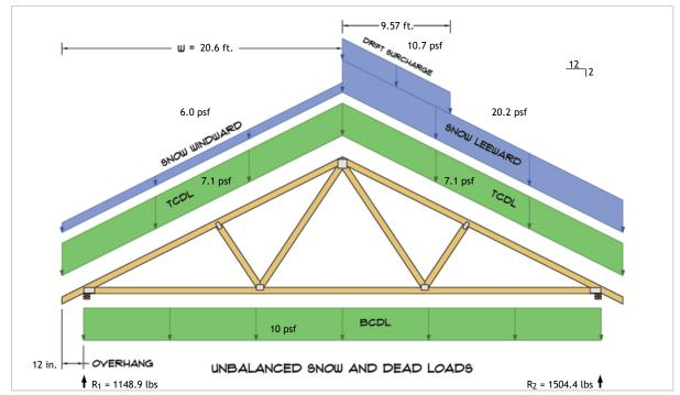
$R_1 = D + S = 684.4 \text{ lbs} + 464.5 \text{ lbs}$  $R_2 = D + S = 684.4 \text{ lbs} + 820.0 \text{ lbs}$
