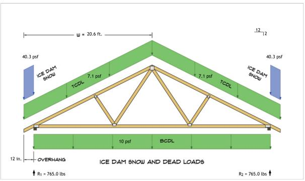
$R_1 = D + S = 684.4 \text{ lbs} + 80.6 \text{ lbs}$  $R_2 = D + S = 684.4 \text{ lbs} + 80.6 \text{ lbs}$
