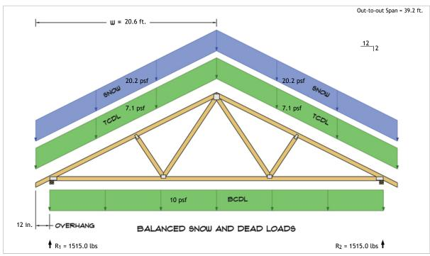
$$\begin{split} R_1 &= D + S = 684.4 \text{ lbs} + 830.6 \text{ lbs} \\ R_2 &= D + S = 684.4 \text{ lbs} + 830.6 \text{ lbs} \end{split}$$
