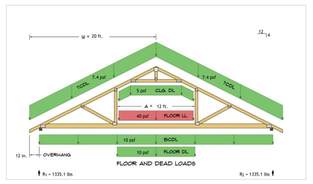
$\begin{aligned} R_1 &= D + L = 855.1 \text{ lbs} + 480.0 \text{ lbs} \\ R_2 &= D + L = 855.1 \text{ lbs} + 480.0 \text{ lbs} \end{aligned}$
