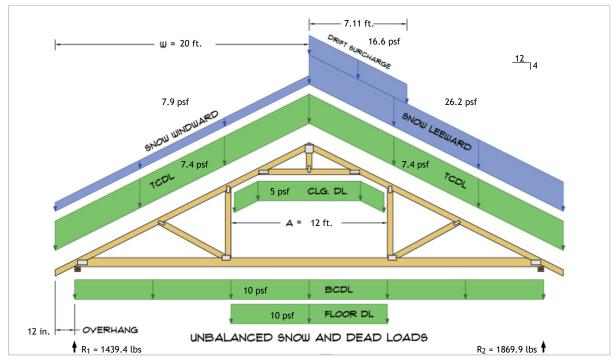
$R_1 = D + S = 855.1 \text{ lbs} + 584.3 \text{ lbs}$  $R_2 = D + S = 855.1 \text{ lbs} + 1014.7 \text{ lbs}$
