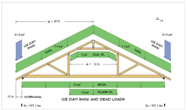
$$\begin{split} R_1 &= D + S = 855.1 \text{ lbs} + 122.0 \text{ lbs} \\ R_2 &= D + S = 855.1 \text{ lbs} + 122.0 \text{ lbs} \end{split}$$
