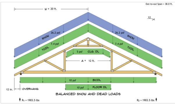
$\begin{aligned} R_1 &= D + S = 855.1 \text{ lbs} + 1048.3 \text{ lbs} \\ R_2 &= D + S = 855.1 \text{ lbs} + 1048.3 \text{ lbs} \end{aligned}$
