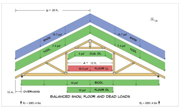
$$\begin{split} R_1 &= D + 0.75L + 0.75S = 855.1 \text{ lbs} + 360.0 \text{ lbs} + 786.2 \text{ lbs} \\ R_2 &= D + 0.75L + 0.75S = 855.1 \text{ lbs} + 360.0 \text{ lbs} + 786.2 \text{ lbs} \end{split}$$
