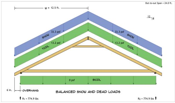
$R_1 = D + S = 220.3 \text{ lbs} + 554.6 \text{ lbs}$  $R_2 = D + S = 220.3 \text{ lbs} + 554.6 \text{ lbs}$
