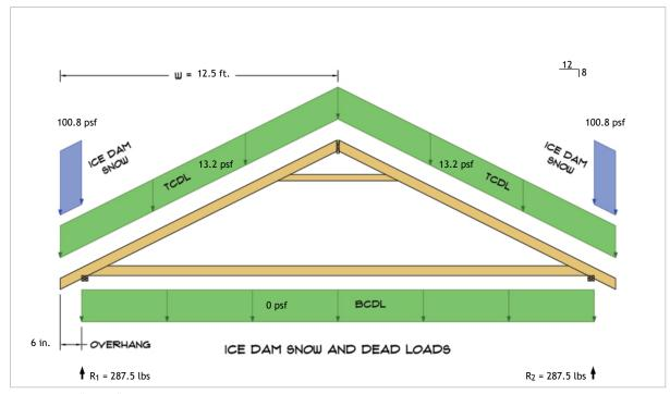
$R_1 = D + S = 220.3 \text{ lbs} + 67.2 \text{ lbs} \\ R_2 = D + S = 220.3 \text{ lbs} + 67.2 \text{ lbs}$
