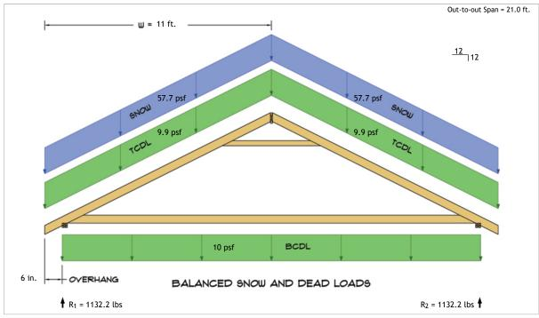
$R_1 = D + S = 285.2 \text{ lbs} + 847.0 \text{ lbs}$  $R_2 = D + S = 285.2 \text{ lbs} + 847.0 \text{ lbs}$
