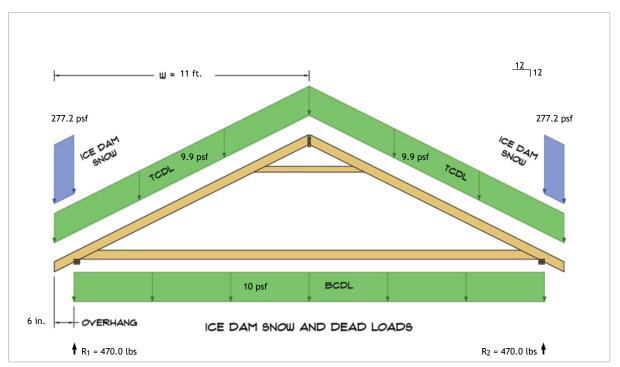
$R_1 = D + S = 285.2 \text{ lbs} + 184.8 \text{ lbs}$  $R_2 = D + S = 285.2 \text{ lbs} + 184.8 \text{ lbs}$
