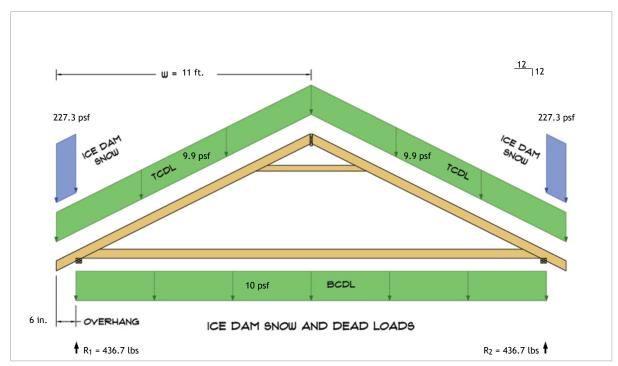
$R_1 = D + S = 285.2 \text{ lbs} + 151.5 \text{ lbs}$  $R_2 = D + S = 285.2 \text{ lbs} + 151.5 \text{ lbs}$
