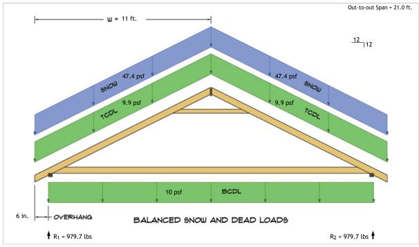
$R_1 = D + S = 285.2 \text{ lbs} + 694.5 \text{ lbs}$  $R_2 = D + S = 285.2 \text{ lbs} + 694.5 \text{ lbs}$
