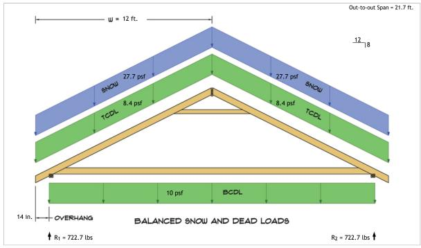
$R_1 = D + S = 279.1 \text{ lbs} + 443.6 \text{ lbs}$  $R_2 = D + S = 279.1 \text{ lbs} + 443.6 \text{ lbs}$
