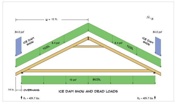
$$\begin{split} R_1 &= D + S = 279.1 \text{ lbs} + 130.7 \text{ lbs} \\ R_2 &= D + S = 279.1 \text{ lbs} + 130.7 \text{ lbs} \end{split}$$
