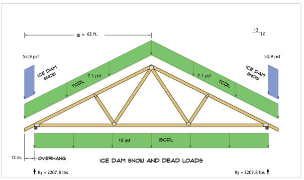
$$\begin{split} R_1 &= D + S = 2100.0 \text{ lbs} + 107.8 \text{ lbs} \\ R_2 &= D + S = 2100.0 \text{ lbs} + 107.8 \text{ lbs} \end{split}$$
