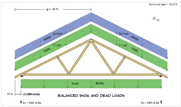
$$\begin{split} R_1 &= D + S = 2100.0 \text{ lbs} + 3341.8 \text{ lbs} \\ R_2 &= D + S = 2100.0 \text{ lbs} + 3341.8 \text{ lbs} \end{split}$$
