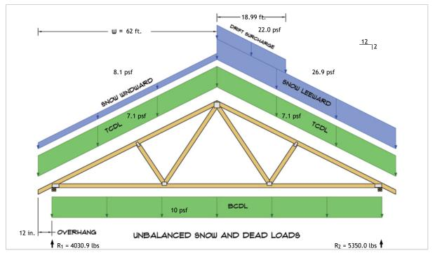
$R_1 = D + S = 2100.0 \text{ lbs} + 1930.9 \text{ lbs}$  $R_2 = D + S = 2100.0 \text{ lbs} + 3250.0 \text{ lbs}$
