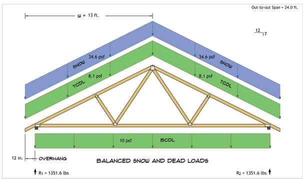
$$\begin{split} R_1 &= D + S = 450.7 \text{ lbs} + 900.9 \text{ lbs} \\ R_2 &= D + S = 450.7 \text{ lbs} + 900.9 \text{ lbs} \end{split}$$
