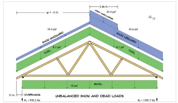
$R_1 = D + S = 450.7 \text{ lbs} + 527.5 \text{ lbs}$  $R_2 = D + S = 450.7 \text{ lbs} + 942.0 \text{ lbs}$
