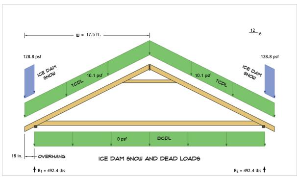
$R_1 = D + S = 234.8 \text{ lbs} + 257.6 \text{ lbs}$  $R_2 = D + S = 234.8 \text{ lbs} + 257.6 \text{ lbs}$
