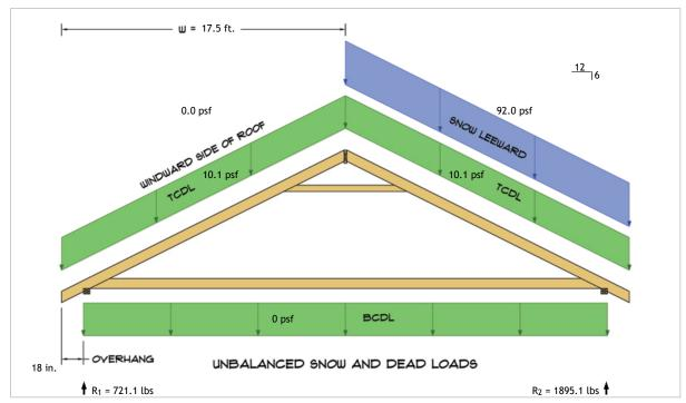
$R_1 = D + S = 234.8 \text{ lbs} + 486.4 \text{ lbs}$  $R_2 = D + S = 234.8 \text{ lbs} + 1660.3 \text{ lbs}$
