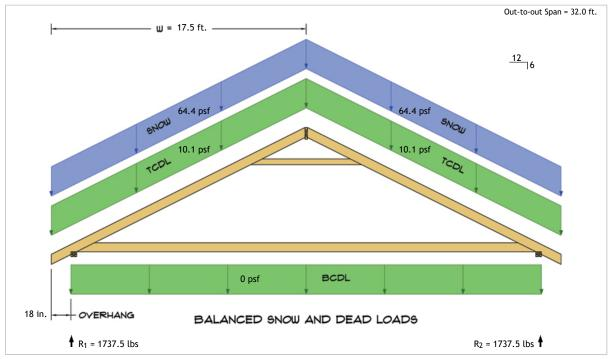
$R_1 = D + S = 234.8 \text{ lbs} + 1502.7 \text{ lbs}$  $R_2 = D + S = 234.8 \text{ lbs} + 1502.7 \text{ lbs}$
