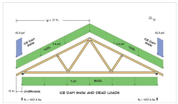
$$\begin{split} R_1 &= D + S = 869.6 \text{ lbs} + 168.0 \text{ lbs} \\ R_2 &= D + S = 869.6 \text{ lbs} + 168.0 \text{ lbs} \end{split}$$
