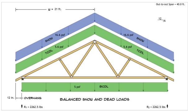
$$\begin{split} R_1 &= D + S = 869.6 \text{ lbs} + 1392.9 \text{ lbs} \\ R_2 &= D + S = 869.6 \text{ lbs} + 1392.9 \text{ lbs} \end{split}$$
