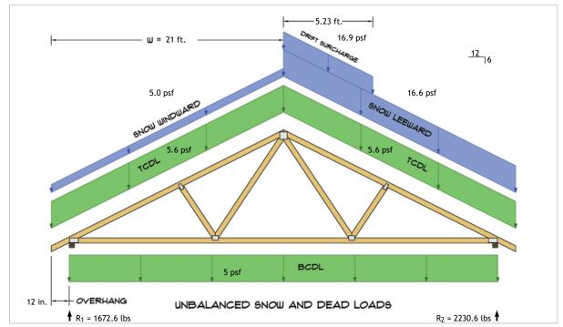
$R_1 = D + S = 869.6 \text{ lbs} + 803.0 \text{ lbs}$  $R_2 = D + S = 869.6 \text{ lbs} + 1361.0 \text{ lbs}$
