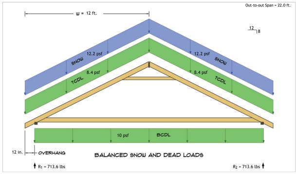
$R_1 = D + S = 421.9 \text{ lbs} + 291.7 \text{ lbs}$  $R_2 = D + S = 421.9 \text{ lbs} + 291.7 \text{ lbs}$
