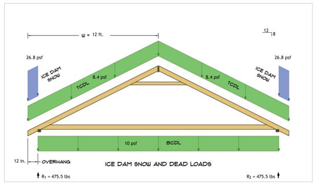
$R_1 = D + S = 421.9 \text{ lbs} + 53.5 \text{ lbs}$  $R_2 = D + S = 421.9 \text{ lbs} + 53.5 \text{ lbs}$
