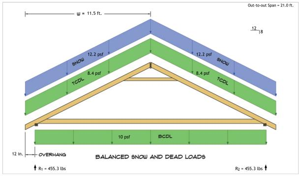
$R_1 = D + S = 269.0 \text{ lbs} + 186.3 \text{ lbs}$  $R_2 = D + S = 269.0 \text{ lbs} + 186.3 \text{ lbs}$
